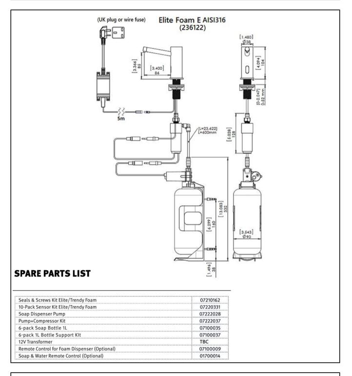
Note: In order to locate the relevant spare part, please check the corresponding parts and part mumber in the drawing. Minimum order quantity will be required.
